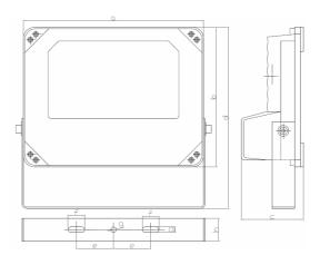
a: 221mm b: 172mm c: 90mm d: 232mm e: 54mm f: 24mm g: 8mm h: 33mm
